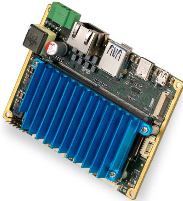
Fig. 1 NXP i.MX8 Reference Design, 2-Channel MIPI CSI-2 Carrier Board with i.MX 8M Plus 4 GB SoM
