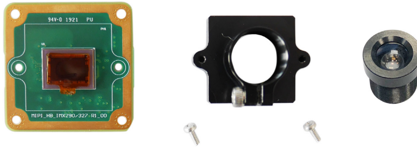
Fig. 10: Sensor, lens holder with screws and lens.
