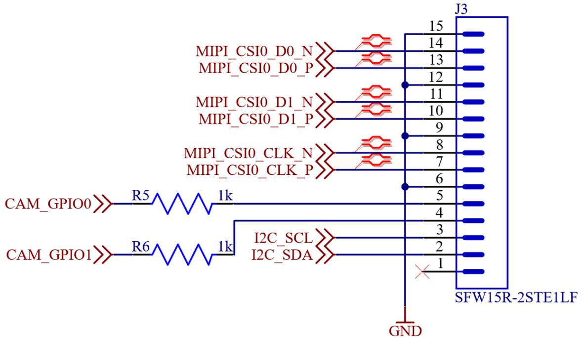
The CAM\_GPIOs and I2C-bus signals have the I/O voltage of 3.3V.
